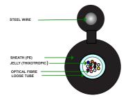
Loose tube containing optical fibres jelly filled are centrally located. A single FRP and single / bunch of Steel Wire are sheathed with core to make figure – 8 constructions for aerial installation.
